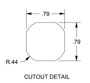
DESCRIPTION: QUARTER TURN, SANITARY, EXTERNAL CAM STOP, 28MM AND 6MM CAM INCLUDED. STAINLESS STEEL TYPE 304
