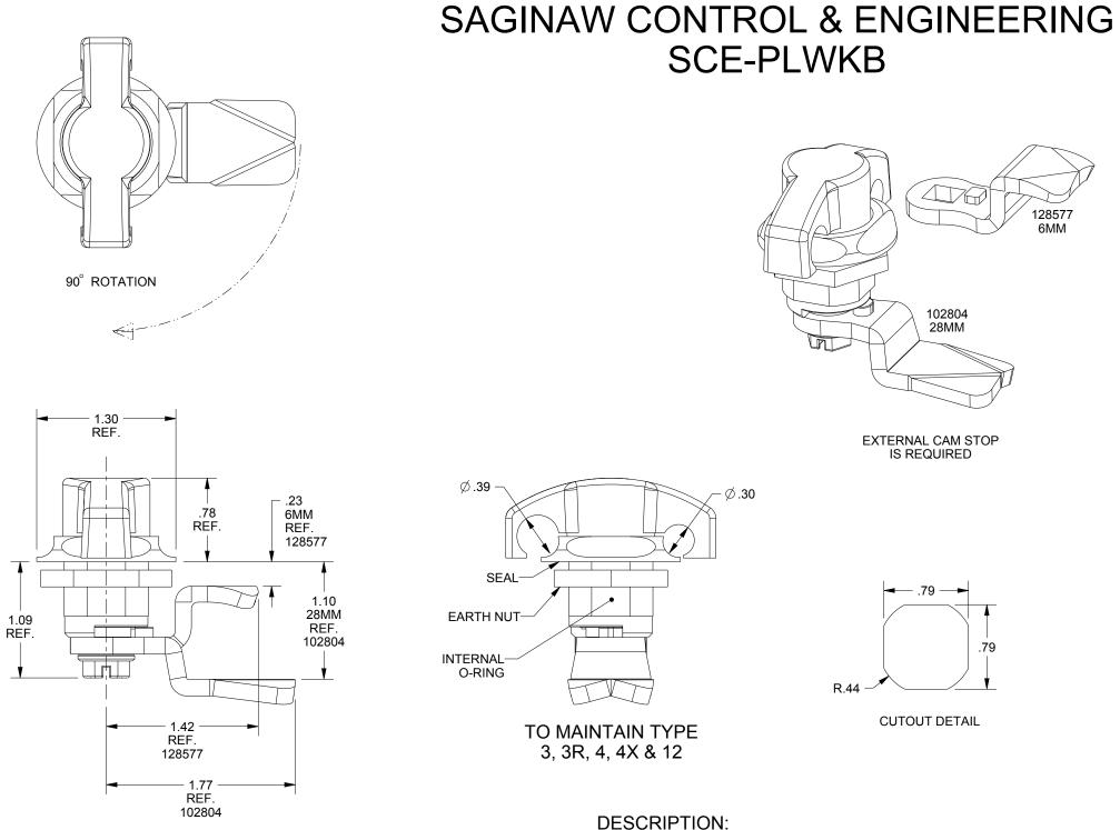
QUARTER TURN, WING KNOB, PADLOCKABLE, EXTERNAL CAM STOP WITH BOTH A 28MM AND A 6MM CAM INCLUDED. ZINC DIE CAST, BLACK TEXTURED
