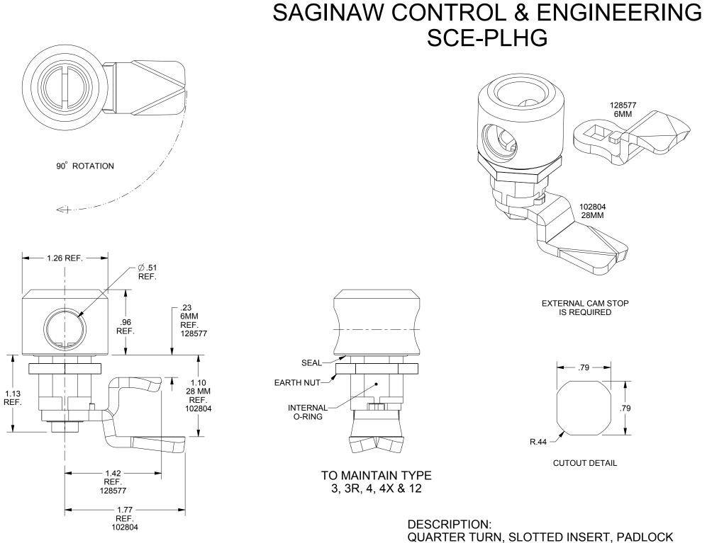
HOUSING, EXTERNAL CAM STOP, 28MM AND 6MM CAM INCLUDED. ZINC DIE CAST, BLACK TEXTURED.
