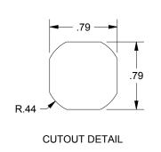
DESCRIPTION: T-HANDLE, NON-LOCKING, EXTERNAL CAM STOP, W/ 28MM CAM ZINC DIE CAST, CHROME PLATED
