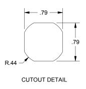
DESCRIPTION: QUARTER TURN, SLOTTED INSERT, EXTERNAL CAM STOP, 28MM AND 6MM CAM INCLUDED. STAINLESS STEEL TYPE 304
