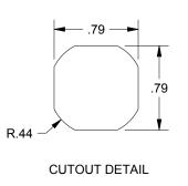
DESCRIPTION: QUARTER TURN, SLOTTED INSERT, OPEN POSITION, EXTERNAL CAM STOP, 28MM AND 6MM CAM INCLUDED. ZINC DIE CAST, BLACK TEXTURED
