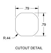
DESCRIPTION: QUARTER TURN, 8 MM SQUARE INSERT W/ KEY, EXTERNAL CAM STOP, 28MM AND 6MM CAMS INCLUDED. ZINC DIE CAST, BLACK TEXTURED
