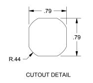
DESCRIPTION: QUARTER TURN, 7 MM TRIANGULAR INSERT W/ KEY, EXTERNAL CAM STOP, CAM INCLUDED 28 MM. ZINC DIE CAST, CHROME
