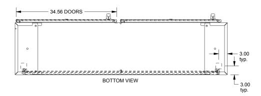
WASH SYSTEM 2" SQUARE DRAIN HOLES IN THE BOTTOM WITH UL APPROVED HOLE SEALS PROVIDED
