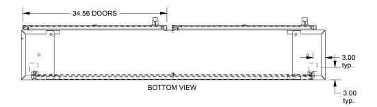
WASH SYSTEM 2" SQUARE DRAIN HOLES IN THE BOTTOM WITH UL APPROVED HOLE SEALS PROVIDED
