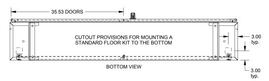
WASH SYSTEM 2" SQUARE DRAIN HOLES IN THE BOTTOM WITH UL APPROVED HOLE SEALS PROVIDED
