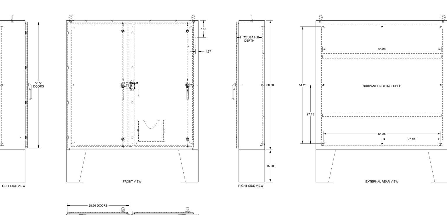
WASH SYSTEM 2" SQUARE DRAIN HOLES IN THE BOTTOM WITH UL APPROVED HOLE SEALS PROVIDED
