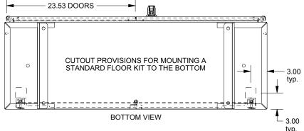
WASH SYSTEM 2" SQUARE DRAIN HOLES IN THE BOTTOM WITH UL APPROVED HOLE SEALS PROVIDED
