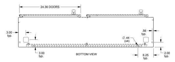
CUTOUT PROVISIONS IN THE BOTTOM AND IN THE REAR WALL FOR SECURING OPTIONAL HEAVY DUTY WALL MOUNTING BRACKET KIT SCE-HDWMK
