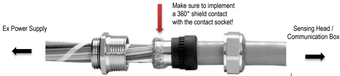
Figure 44: EMC Compliant Connection for the Cables for Sensing Heads and Communication Box
