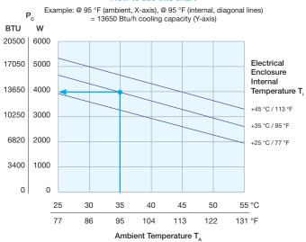
Note: Cooling capacity may vary between voltage and configurations.
