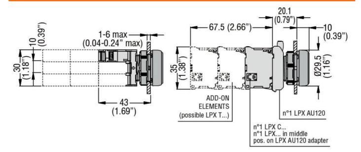
LED INTEGRATED LAMP-HOLDER, STEADY LIGHT Ø22MM PLATINUM SERIES, SCREW TERMINATION, 185...265VAC. YELLOW
