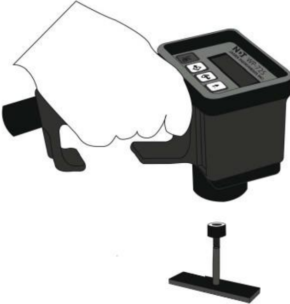
Figure 18: Placing the Measuring Micrometer on the Gauge Plate
