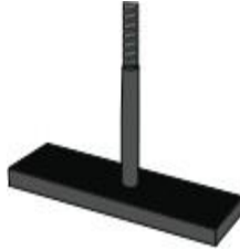
Figure 16: Leveling the Measuring Plate with the Concrete Surface
