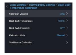
Aim the device at the black body and press **OK** to complete calibration.
