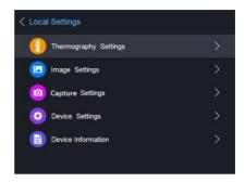
Set thermography range, emissivity, distance, background temperature, reflection temperature, humidity, and black body temperature calibration.
