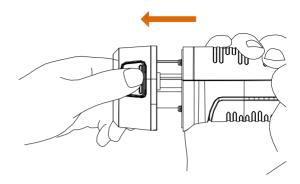
Insert the battery into the charging base. See figure below.
