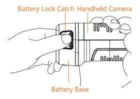
2. Hold the lock catches, and draw the battery base to take out the battery. See figure below.
