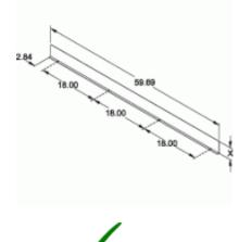
• Divides wireway into two or more compartments. Barriers are fastened to wireway sections with screws.
