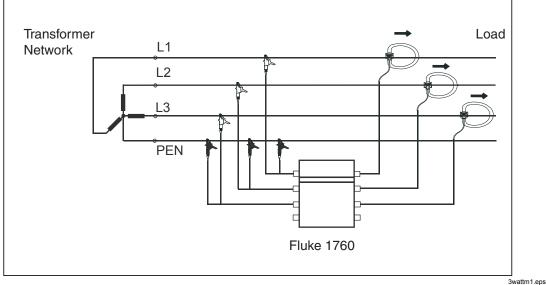
Figure 3-4. Circuit Diagram: 4-Wire Network (Wye Connection)
