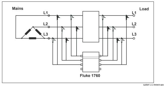
Figure 3-7. Circuit Diagram: 2 Voltage System in Delta Connection
