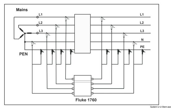
Figure 3-6. Circuit Diagram: 2 Voltage System with Neutral
