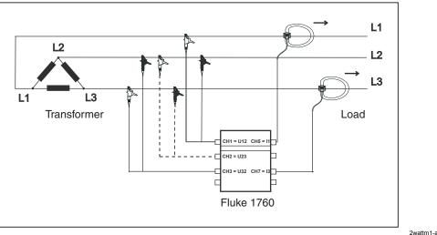
Figure 3-2. Circuit Diagram: 3-Wire Network (Aron 2)
