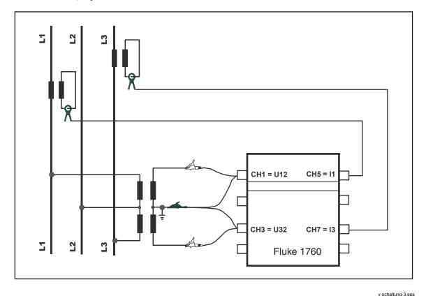
Figure 3-3. Circuit Diagram: Aron 2 Method/Open Delta Method
