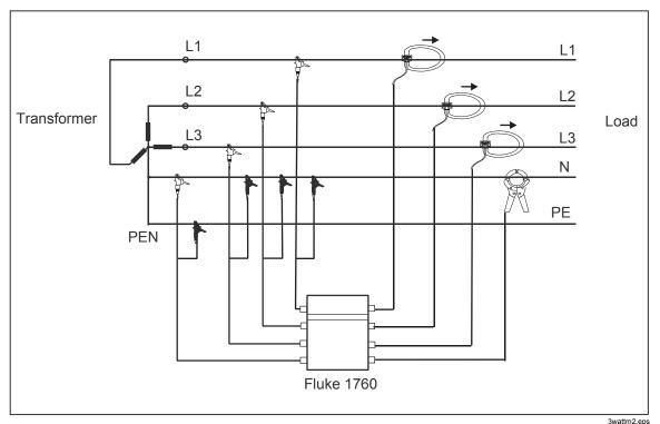
Figure 3-5. Circuit Diagram: 4-Wire
