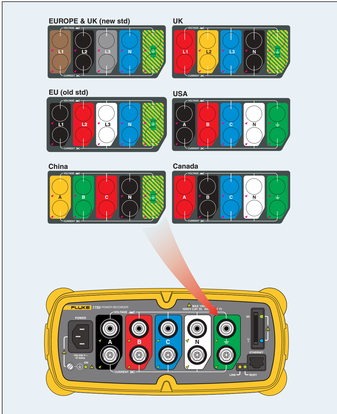
Figure 2. Applying the Front Panel Decal
