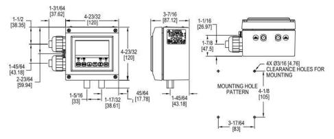
The Series DHII Digihelic® II Differential Pressure Controller takes all the features of the standard Digihelic® pressure controller and packages them in a robust NEMA 4 (IP66) housing.
