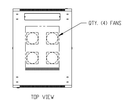
MATERIAL: PANEL MOUNTING RAILS - 14 GA. (0.08" [2.0] THK.) STEEL ALL OTHER PARTS - 18 GA. (0.05" [1.2] THK.) STEEL
