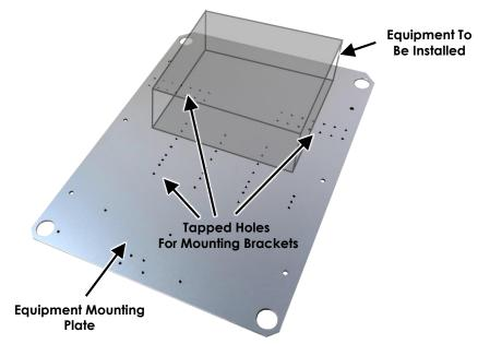
2. Once the location of the (3) equipment mounting brackets are determined, secure each to the equipment mounting plate using the supplied screws.
