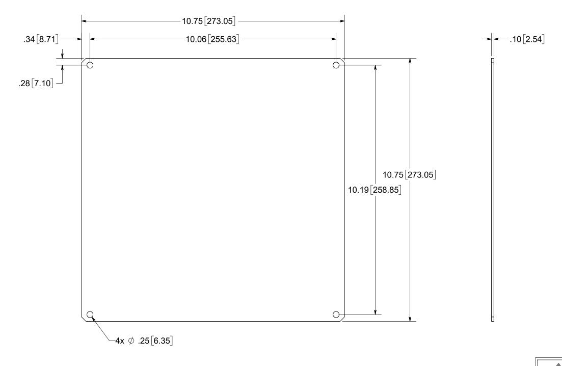
**ALUMINUM 300-H14** WITH PROTECTIVE PEEL-OFF FILM ON ONE SIDE
