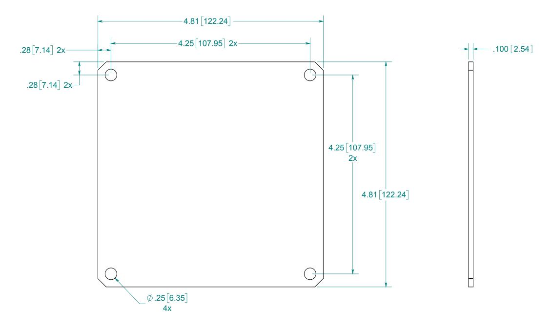
ALUMINUM 3003-H14 WITH PROTECTIVE PEEL-OFF FILM ON ONE SIDE.
