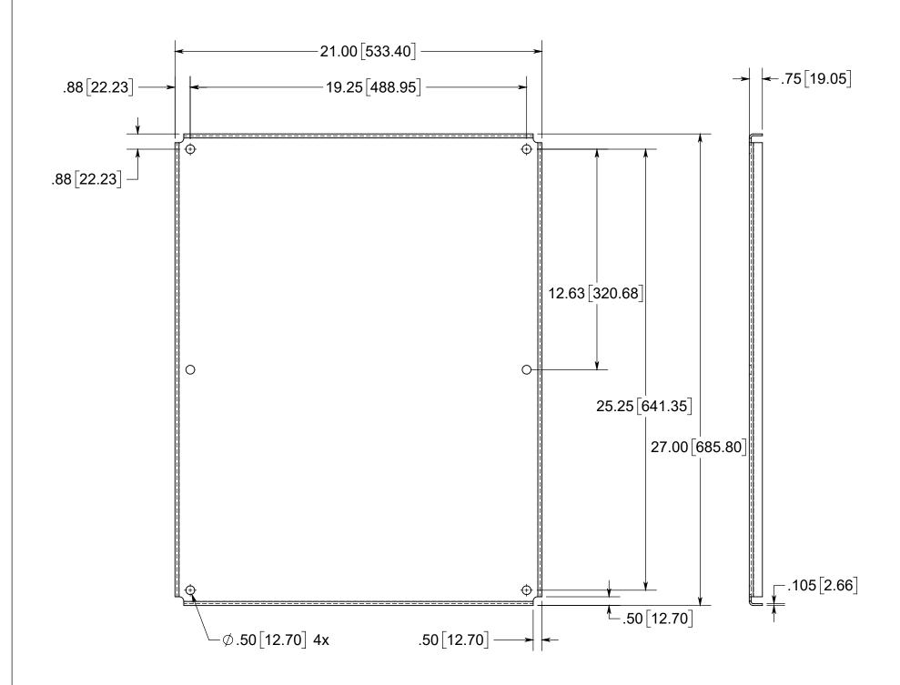
Galvannealed Steel 14 Gauge
