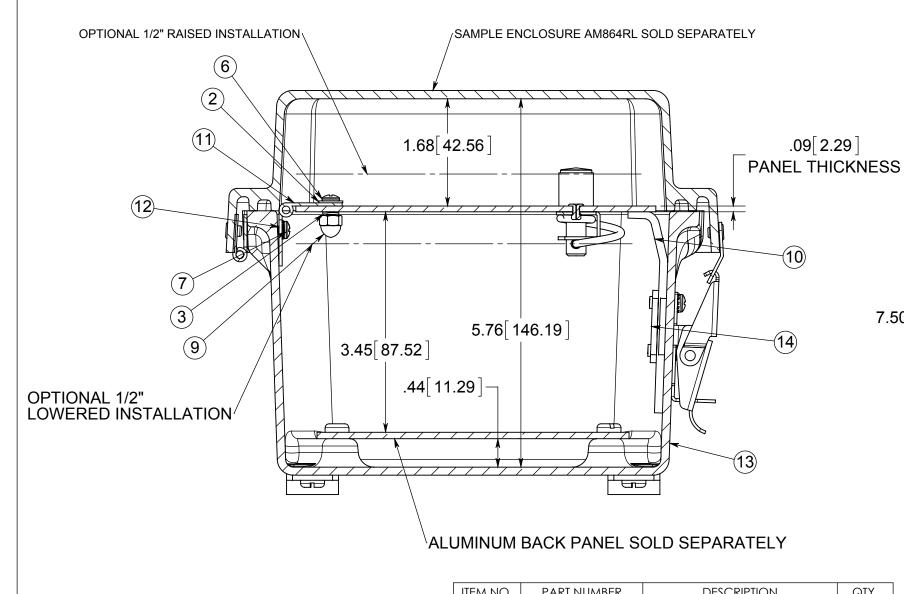
NOT ALL PARTS OF THE HFP ASSEMBLY KIT ARE SHOWN, ONLY THE PARTS USED IN THE FLUSH INSTALLATION OF THE PANEL. FOLLOW INSTALLATION INSTRUCTIONS INCLUDED IN THE KIT FOR THE OPTIONAL PANEL MOUNTING.
