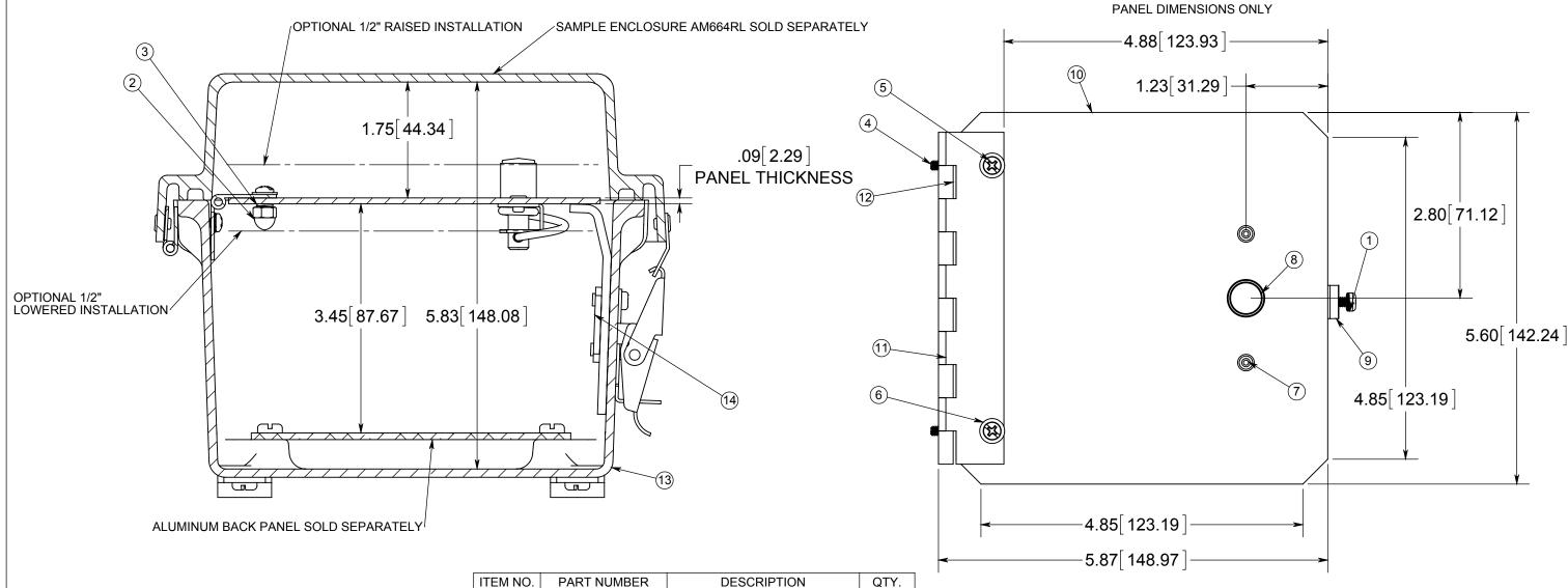
NOT ALL PARTS OF THE HFP ASSEMBLY KIT ARE SHOWN, ONLY THE PARTS USED IN THE FLUSH INSTALLATION OF THE PANEL.
