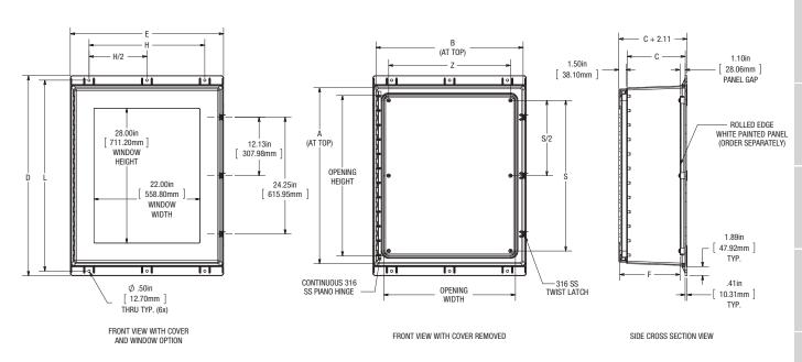
H/2 [ 711.20mm ] WINDOW HEIGHT 22.00in 558.80mm 1 WINDOW Ø .50in [ 12.70mm ]
