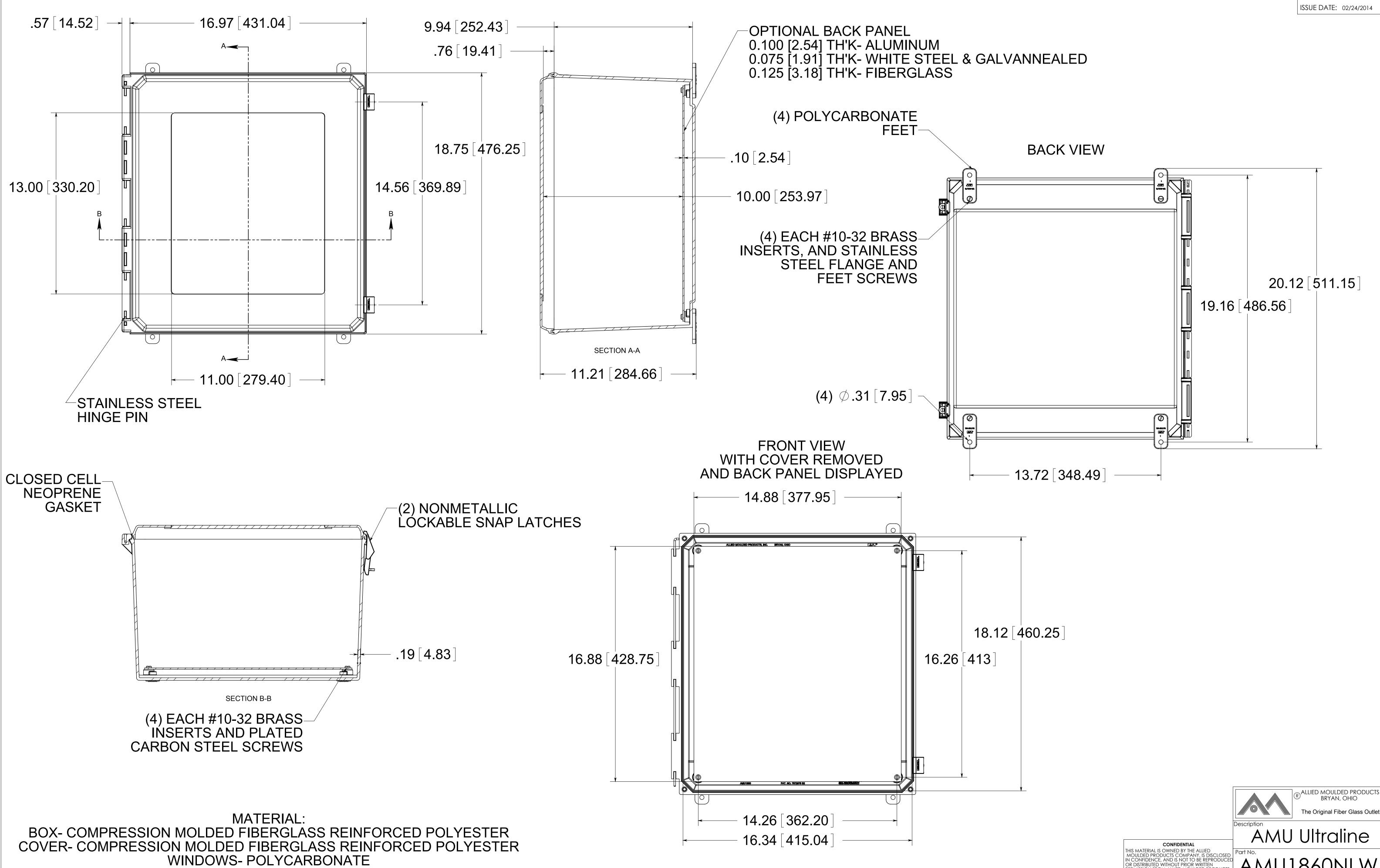
The Original Fiber Glass Outlet Bo AMU Ultraline CONFIDENTIAL THIS MATERIAL IS OWNED BY THE ALLIED MOULDED PRODUCTS COMPANY, IS DISCLOSED IN CONFIDENCE, AND IS NOT TO BE REPRODUCED OR DISTRIBUTED WITHOUT PRIOR WRITTEN PERMISSION FROM ALLIED MOULDED PRODUCTS. AMU1860NLW
