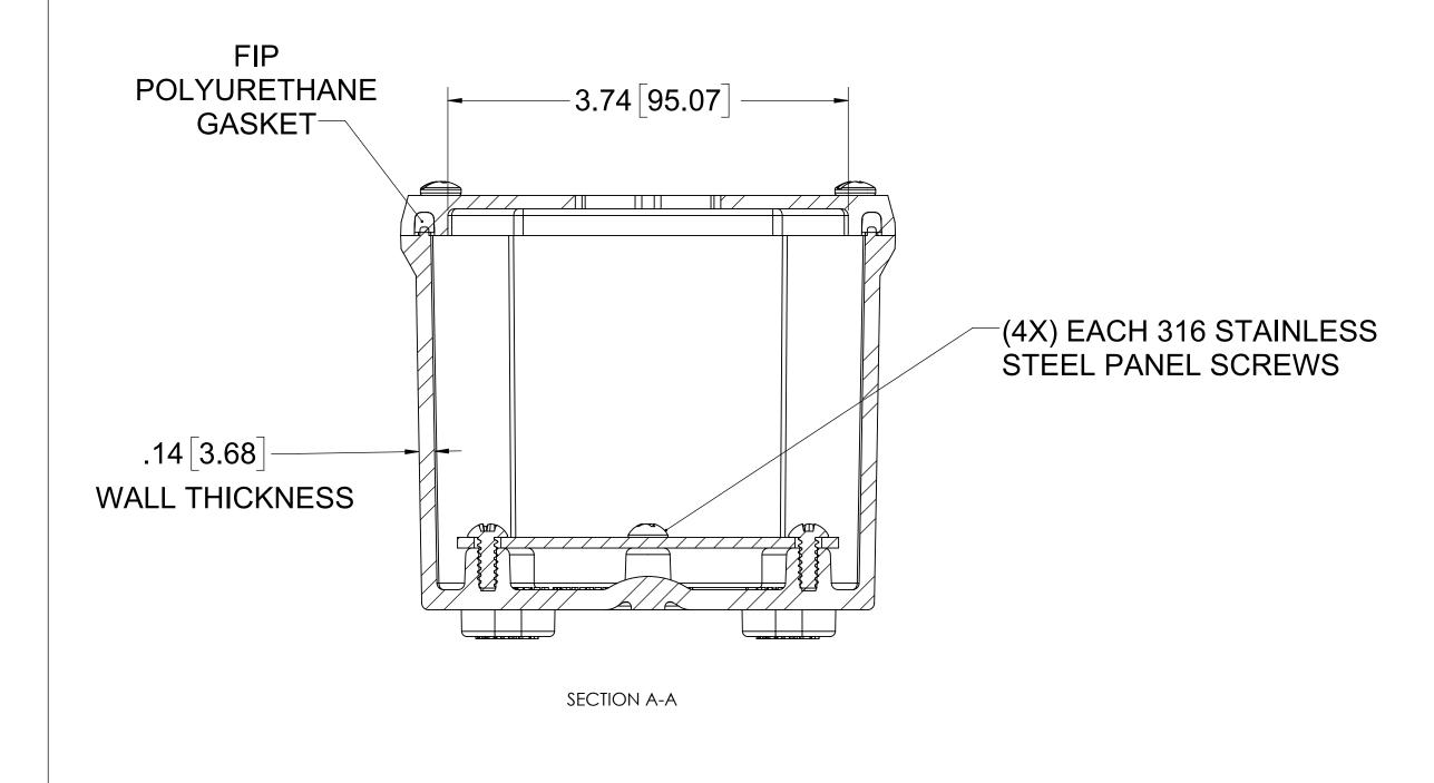
MATERIAL: BOX - INJECTED POLYCARBONATE STANDARD COVER - INJECTED POLYCARBONATE CLEAR COVER - INJECTED POLYCARBONATE
