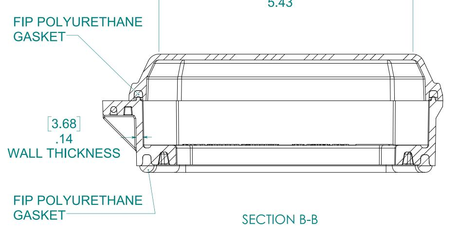
**MATERIAL**: FRAME- INJECTED POLYCARBONATE STANDARD COVER- INJECTED POLYCARBONATE CLEAR COVER- INJECTED POLYCARBONATE
